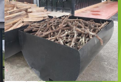
Retort kiln Fusion Experience Ltd Nairobi. 34% efficiency
