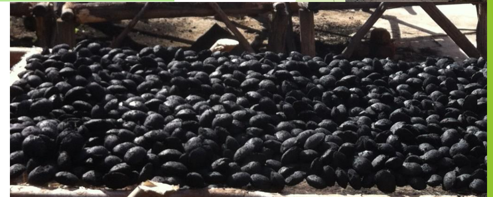
Briquette production from tree branches in drylands
