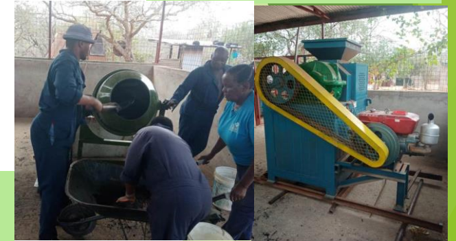
Retort kiln Fusion Experience Ltd Nairobi. 34% efficiency
