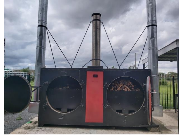
Retort kiln Fusion Experience Ltd Nairobi. 34% efficiency
