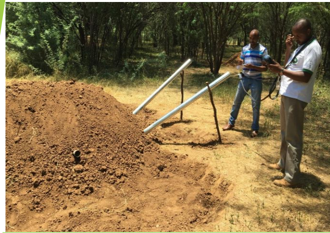
Measuring emissions from improved earth mound kiln (IEK) Photo Mary Njenga 2019
